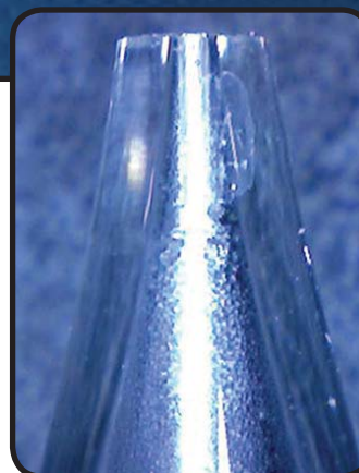
Water microdroplets continuously clean the inside of the nebulizer and prevent salt deposits.
