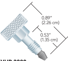
VHP-3200x 10-32 VHP Fitting for 1/16" OD tubing
