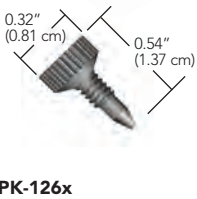
PK-126x 6-32 PK MicroTight® Fitting for 1/32" OD tubing
