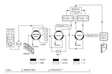
Figure 2: System switching diagram.
